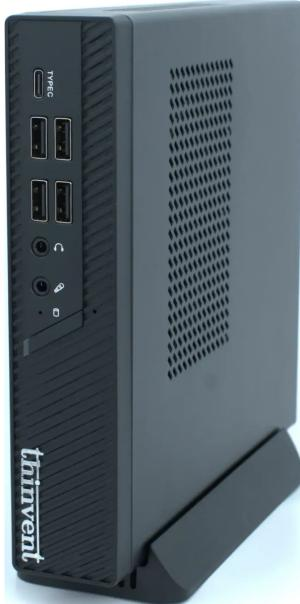
Thinvent® Aero Mini PC, Intel® processor N95 (4 core, up to 3.4 GHz, 6 MB cache), 32GB DDR4 RAM, 32GB MLC SSD, 12V 5A Adapter, No WiFi, Thinux™ Embedded Linux
