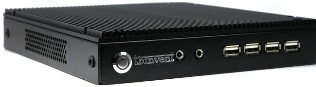
Thinvent® Industrial PC IPC1, Intel® processor N100 (4 core, up to 3.4 GHz, 6 MB cache), 32GB DDR4 RAM, 128GB SSD, 12V 2A Adapter, No WiFi, Thinux™ Embedded Linux
