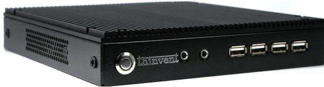
Thinvent® Industrial PC IPC1, Intel® processor N100 (4 core, up to 3.4 GHz, 6 MB cache), 4GB DDR4 RAM, 128GB SSD, 12V 5A Adapter, No WiFi, Thinux™ Embedded Linux
