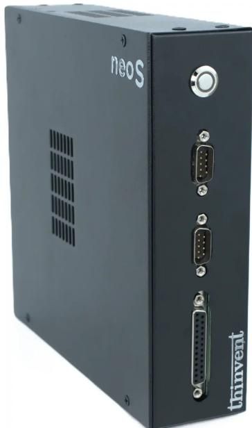
Thinvent® Neo S Thin Client, Intel® processor J4125 (4 core, up to 2.7 GHz, 4 MB cache), 8GB DDR4 RAM, 1TB SSD, 19V 3A Adapter, No WiFi, Thinux™ Embedded Linux, Thinvent® Keyboard and Mouse set
